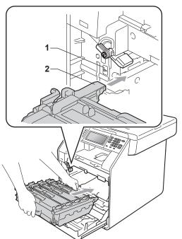
Turn the green lock lever (1) clockwise to the lock position.
